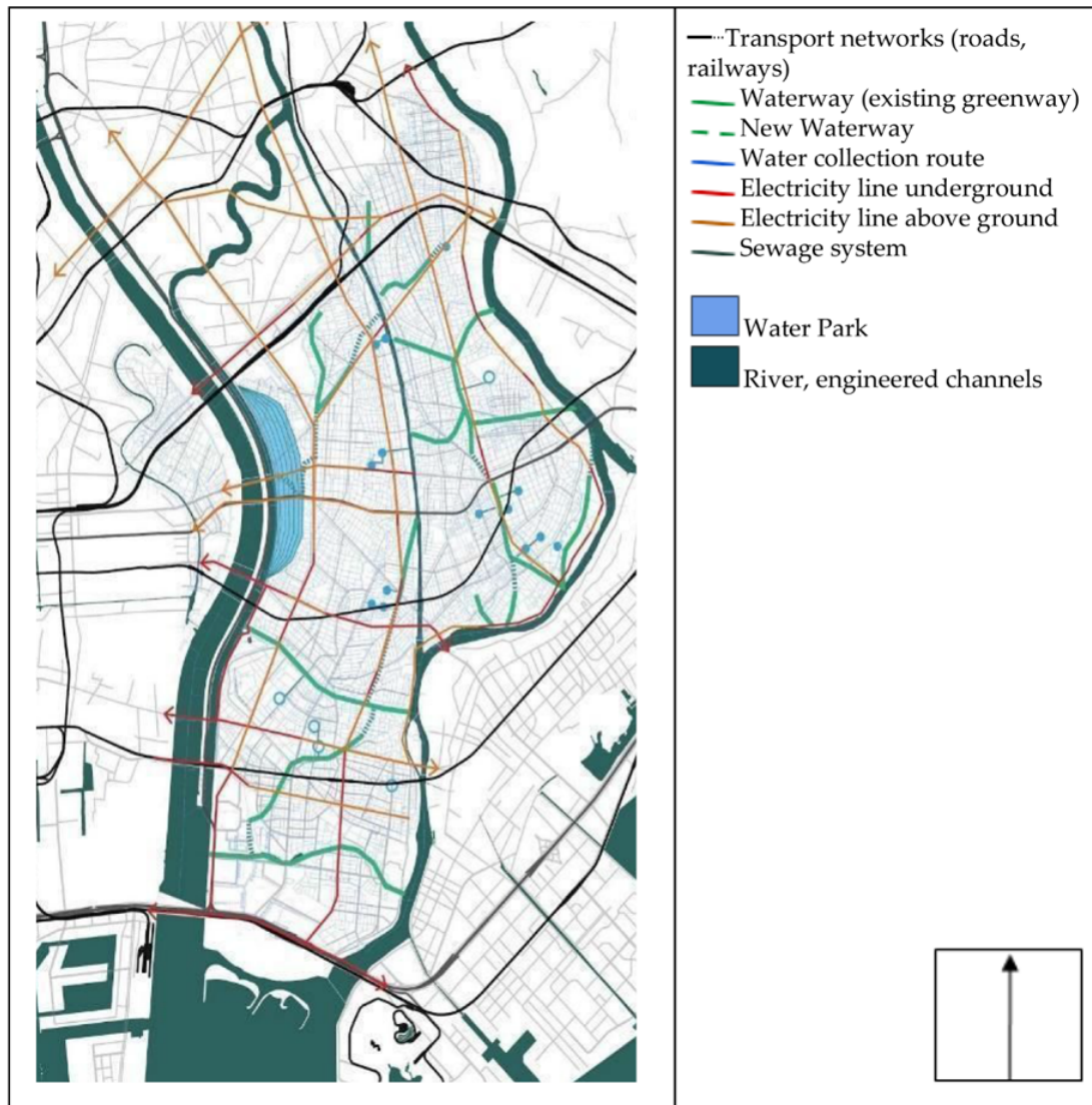
Figure 12. Strategy A—anti super levee overlaid with vital infrastructure (electricity, transport, sewage) (source: drawn using data from MLIT Japan and the Edogawa ward data, 2016) [11,19].
