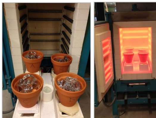
Step 30: Place the set up in the oven, see firing scheme in Chapter 7.
