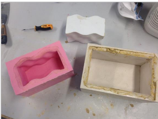
Step 17: Disassemble the casts and remove 3D print.
