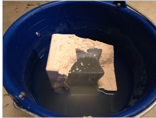
Step 32: Placing the crystal cast in a bucket of water will dissolve the crystal cast.
