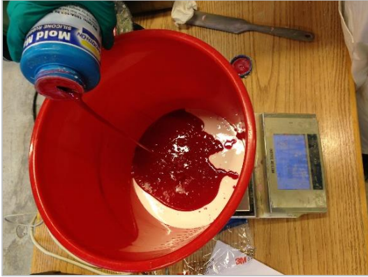
Step 7: Add the two-component silicon mix according to the instructions and make sure to have sufficient mixture to cast on the geometry with a cover of about two centimetres of silicon.
