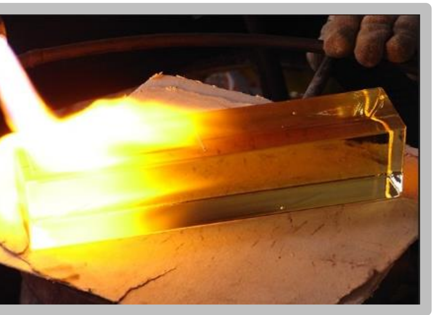
Post-processing of cast glass brickwork applied in the Optical Glass House in Hiroshima, Japan. Reprinted from (Tadashi Oshima, 2012).
