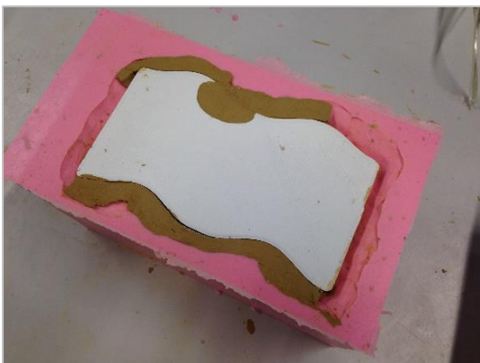
Step 11: Demould, take out the clay but leave the geometry inside the silicone cast. A gypsum cast is needed to restrain the silicon mould for future steps.
