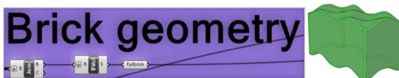
Figure 168: Using boundary volume a solid is generated of the brick geometry.
