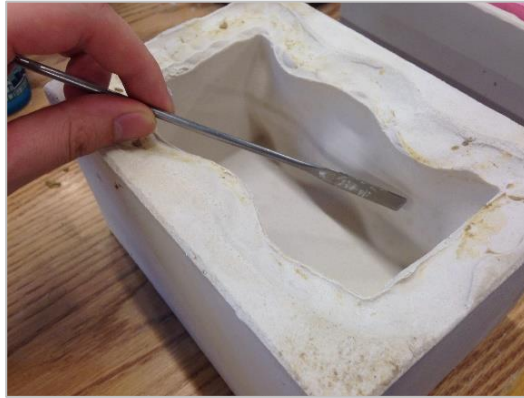
Step 26: Remove any residual wax manually.
