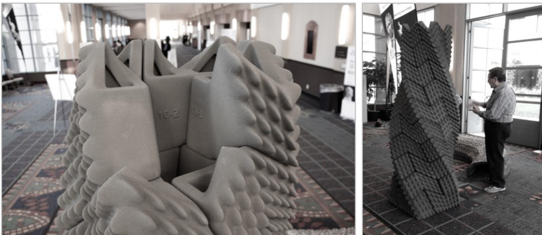
Figure 25: Interlocking 3D printed elements, designed to withstand earthquake based on Inca masonry interlocking systems. The slight in-plane angle combined with the interlocking system and no mortar interlayer increases the structural resistance against earthquakes. Reprinted from (MacLeod, 2014).
