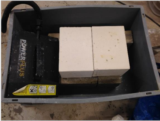
Step 25: Place the crystal cast in a steaming set up To melt the wax from the crystal cast.
