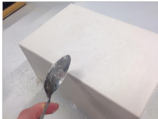
Step 16: Remove sharp edges with a spoon to prevent easy breakage of the cast.
