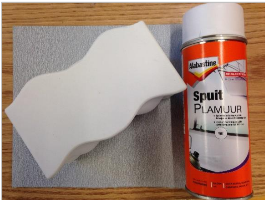
Step 3: Filler is applied to smoothen the 3D printed geometry. Otherwise 3D printed layering will show in the glass geometry.
