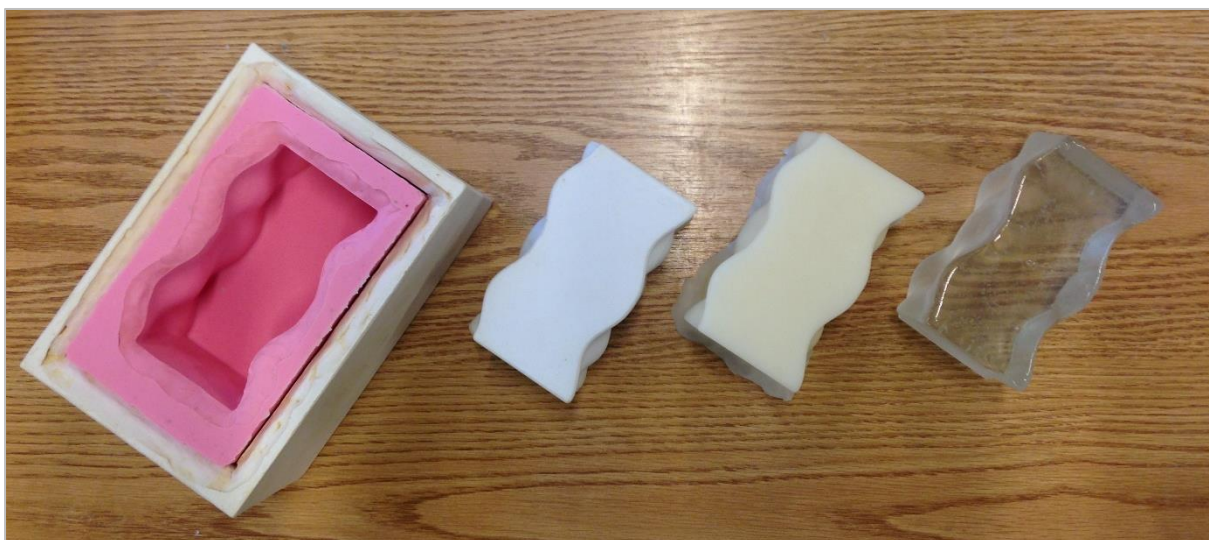
Figure 131: Brick manufacturing stages, from left to right: Silicon negative; 3D printed geometry; wax geometry; resulting glass brick.
