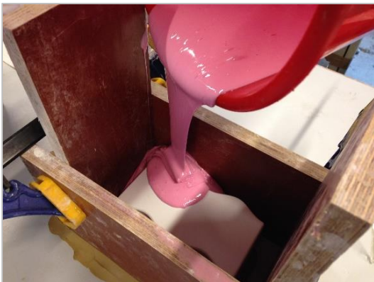
Step 9: Cast the silicone mixture gradually into corner to ensure the geometry is completely covered with silicon and fewer air inclusions.
