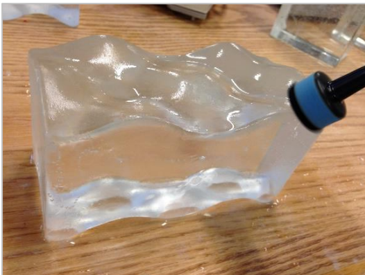
Step 33: Due to impurities and flaws post processing is necessary. Hence the geometry is polished.
