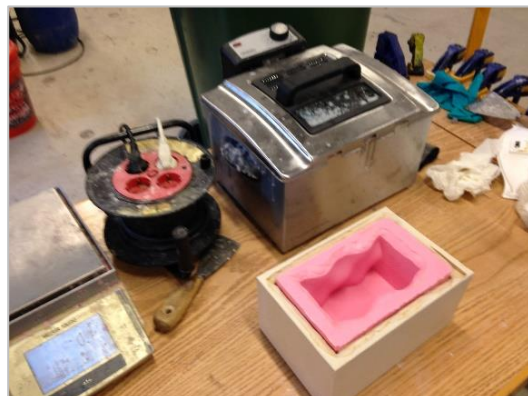
Step 18: Melt wax and place silicon mould in gypsum cast.
