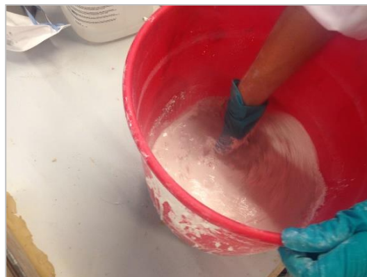
Step 12: Mix water and gypsum (ratio 1:1.75), make sure to make sufficient for covering the silicon mould with about an additional 2 cm thickness.
