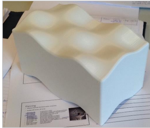
Step 2: 3D print geometry, make sure the printed geometry is a solid. The geometry is printed with a precision of 100 micron and 0.8 nozzle.
