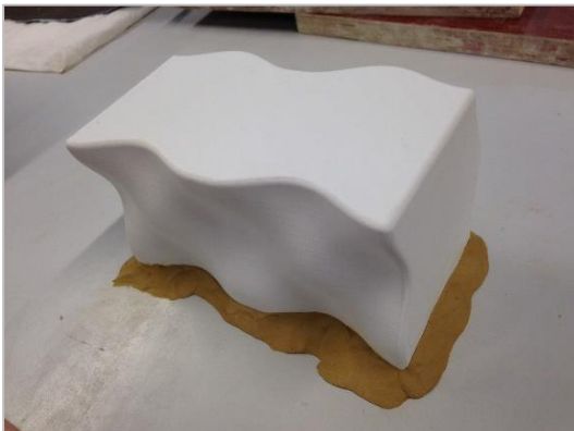
Step 5: Apply a clay edge around the extra added geometry to prevent the silicone mix to flow underneath the 3D printed geometry.
