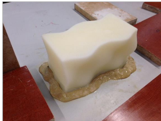
Step 22: Place the wax geometry on a flat surface, and make sure the geometry is level. Apply some clay on the seams and add some soap for easier release of the crystal cast.
