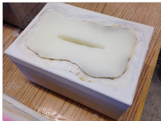
Step 24: After about an hour the moulding can be removed.
