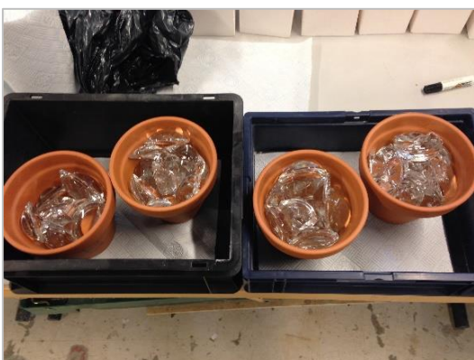
Step 29: Weigh the glass and place into the flower pots for the corresponding moulds. The needed glass weight is determined by measuring the volume of water fitting in the mould and calculating the needed glass mass.
