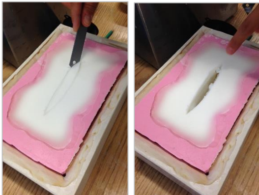
Step 21: For speeding up the process one can apply a cut into the geometry and get rid of the molten wax core. This also prevents some shrinkage of the wax geometry.
