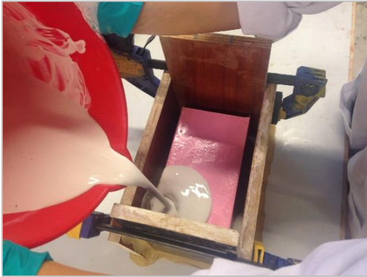
Step 13: Cast the mixture in a corner of the new moulding (all seams again closed with clay).
