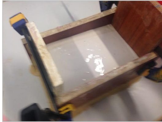
Step 14: Knock to release entrapped bubbles, wait 45 minutes to an hour for hardening.
