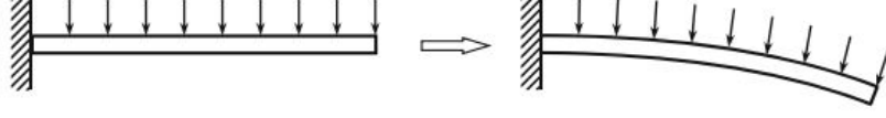
Figure 4.5: The left figure illustrates the initial state of a cantilever beam, while the right figure depicts the beam subjected to a distributed load, highlighting the change in the direction of the follower forces. This figure is obtained from Kim (2015)
