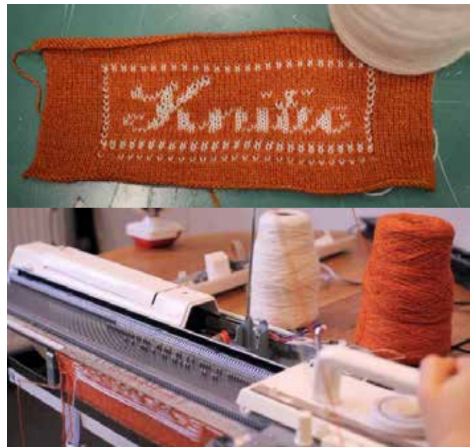
Figure 2. KNITIC digital design knitting machine & pattern example
