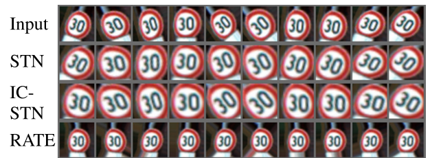
FIGURE 1. Image alignment result on traffic sign dataset. The first row shows variations of a traffic sign image followed by their aligned versions of STN, IC-STN and the proposed RATE shown in the second, third and fourth rows respectively.
