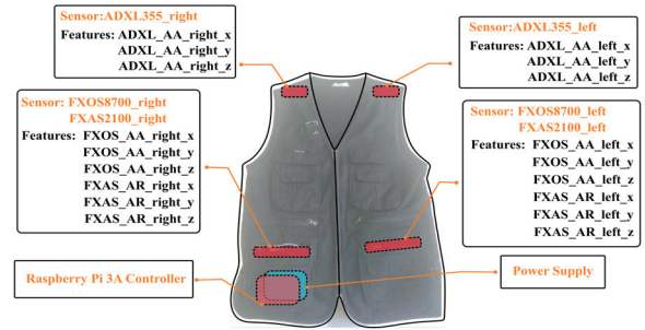
FIGURE 8. The features captured by each sensor and the assembling position of each sensor on the comfort wearable. The same features are captured on the tight-fit wearable, and the sensors are assembled on similar positions.
