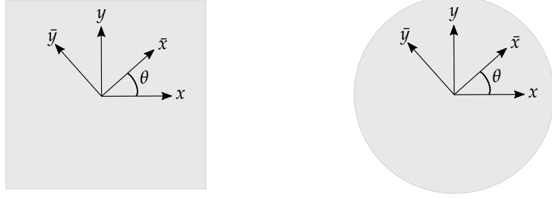
Figure 4.1: Local \bar{x}, \bar{y} -coordinate system rotated with angle \theta with respect to a global x, y -coordinate systems of the square and circular RVE.
