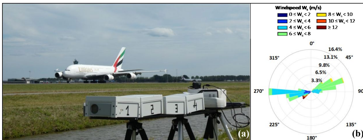
Figure 4.6: Equipment set-up of the co-location experiment (a) and a wind rose showing the percentage of occurrence of the wind approaching from a certain direction together with the wind speed (b)
