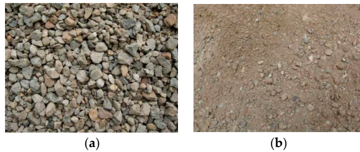
Figure 1. Recycled Aggregates. (a) Recycled Coarse Aggregates (RCA); (b) Recycled Fine Aggregates (RFA).
