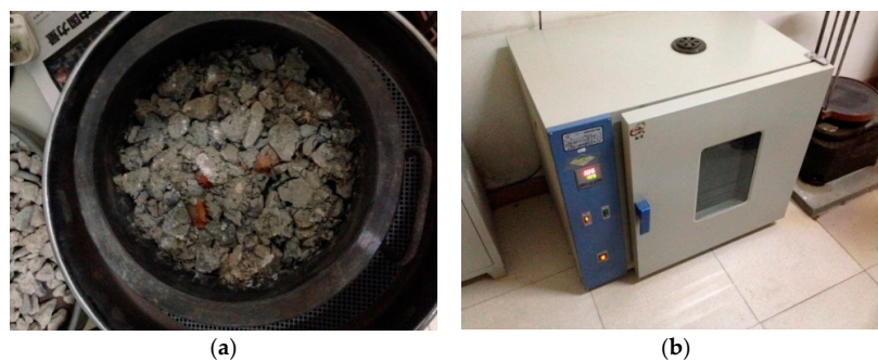
Figure 2. Instruments used for measuring the physical properties of the aggregates. (a) Crush index; (b) Water absorption.
