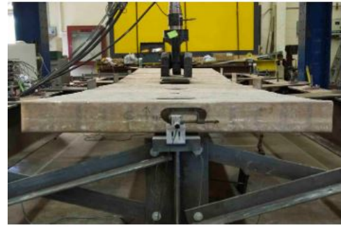
Figure 2.16: Three-point bending specimen from Davalos et al. [27]
