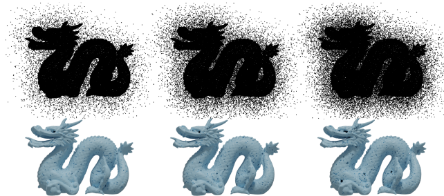
Figure 21: Results of GLOBAL BALLMERGE with from l.t.r.: 10%, 20%, and 30% outliers - \delta = 1.75, 1.7, 1.68 respectively (RMS error w.r.t bbox diagonal: 0.000567, 0.000554, and 0.000793).
