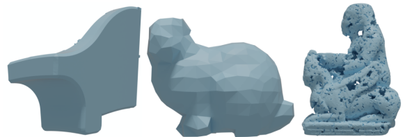
Figure 28: Limit cases (l.t.r.): Sharp edges on artificial object, under-sampled regions (bunny ears) not reconstructed (down-sampled to 1%), and extreme outlier levels (40%).
