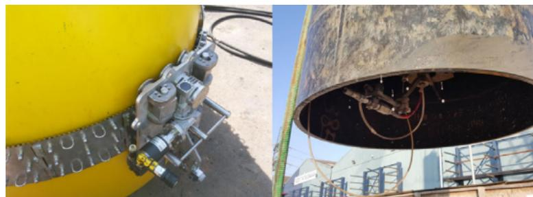
Figure 2.2: Abrasive water jet cutters, left: External Abrasive WaterJet cutter (EAWJ), right: Internal Abrasive WaterJet cutter [19].
