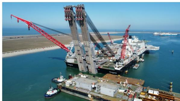
Figure 1.6: The Jacket Lift System on the Pioneering Spirit with its two beams and six main hoist systems with a capacity of 5000 tons each[18]. The total capacity of the JLS is still 20.000 tons, since not all six main hoist systems can operate at maximum capacity at the same time.
