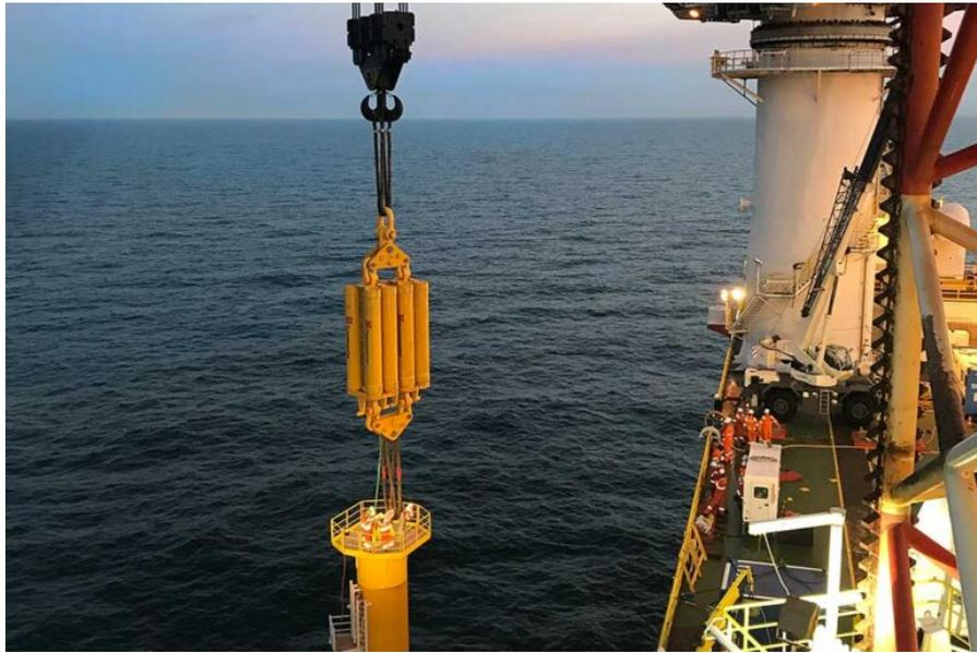
Figure 3.3: Example of a 1200 ton cranesmaster [23].
