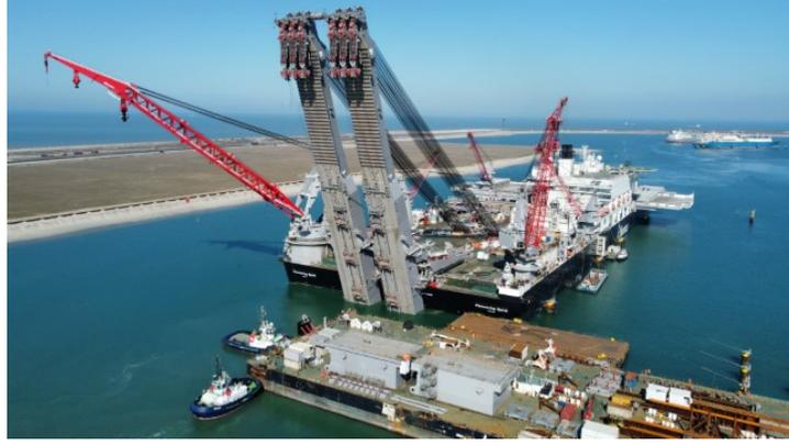
Figure 5.4: The Jacket Lift System on the Pioneering Spirit with its two beams and six main hoist systems with a capacity of 5000 tons each[18]. The total capacity of the JLS is still 20.000 tons, since not all six main hoist systems can operate at maximum capacity at the same time.
