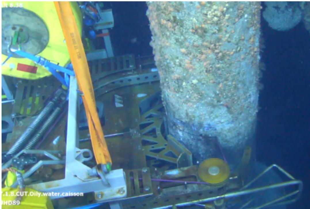
Figure 2.1: A diamond wire cutter in action. The diamond wire that cuts through the pipe is circulating around the pulleys, creating friction between the diamond particles in the wire and the pile itself [18].
