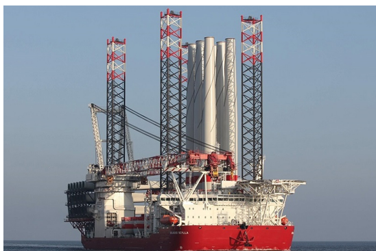
Figure 2.1: Jack-up Seajacks Scylla in transit mode, on its way to a wind farm.
