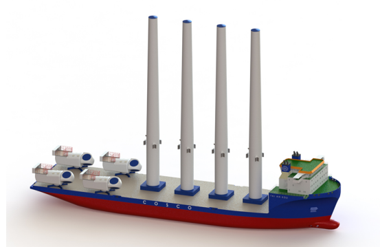
Figure 4.5: Layout 3: Nacelles moved to the sides of the vessel.
