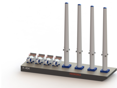
Figure 4.1: Layout 1: Starting deck layout on planar bow barge H-404.
