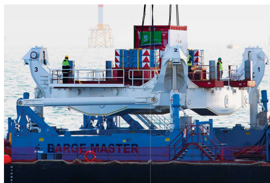
Figure 5.2: Bargemaster's BM-T700 motion compensation system.
