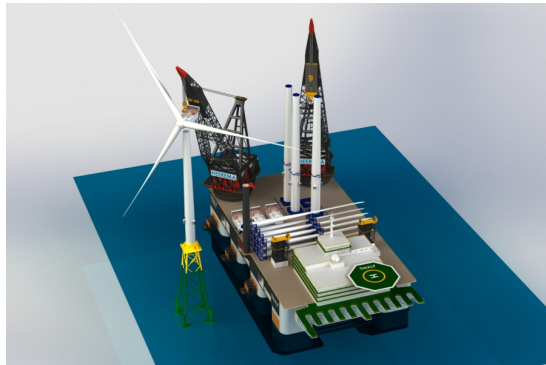
Figure 3.2: Proposed installation method: RNA installation on tower.
