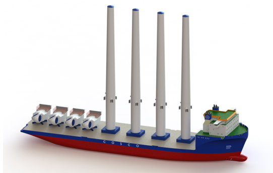
Figure 4.2: Layout 1: Starting deck layout on HTV Tai An Kou.
