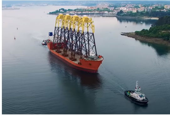
Figure 3.4: Dockwise Swan carrying four jackets.
