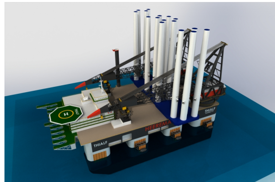
Figure 5.7: Deck layout of the 8T-Frame concept, cranes boomed down.
