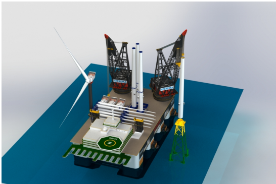
Figure 3.1: Proposed installation method: RNA assembly and tower installation.
