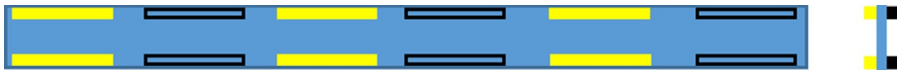
Fig. 7.16 Configuration of the smart corrugated structure. Configuration of the smart corrugated structure with horizontal 4D-printed beams. No permission required.
