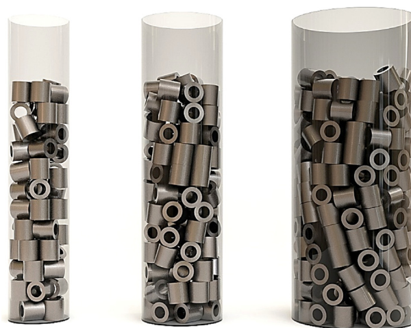
Fig. 1. The RBD-simulated structures of Raschig rings with N_{pv} = 3.06, 4.05, 6.02 .
