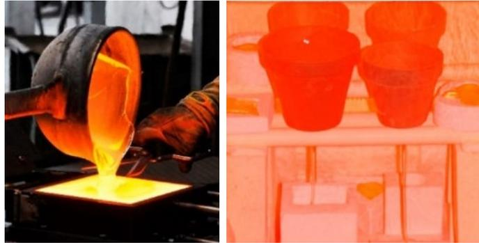
Figure 2.13 Left: primary casting. Right: secondary casting. From (Oikonomopoulou, 2019).
