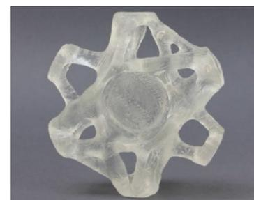
Figure 3.15 Topology optimised cast glass shell node. From (Damen, 2019).
