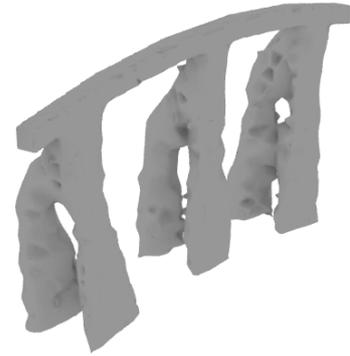
Figure C.4 topology optimised railing
