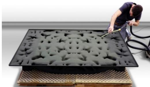
Figure 2.21 Post-processing of the 3D printed sand mould. From (Jipa et al., 2016).
