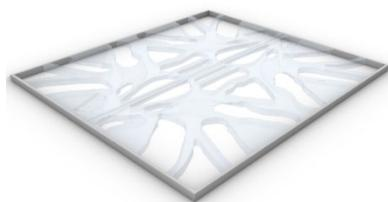
Figure 3.19 Topology optimised cast glass slab. From (Stefanaki, 2020).
