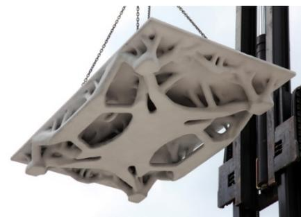
Figure 3.12 Optimised concrete slab prototype B. From (Jipa et al., 2016).
