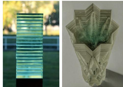
Figure 2.7 Stacked glass columns. Left: Experimental tested column, Right: Artistic impression. From (Heugten, 2013).
