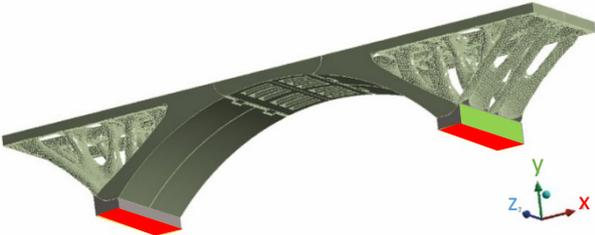
Figure 9.16 Support conditions for non-linear analysis cycle with an elastic supported foundation in the x-direction. Red indicates the restrained surface in the x- and z-direction, and in green, the horizontal elastic support.
