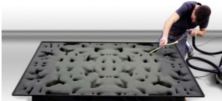
Figure 9.25 Removal of residual sand after printing. From (Jipa et al., 2016).
