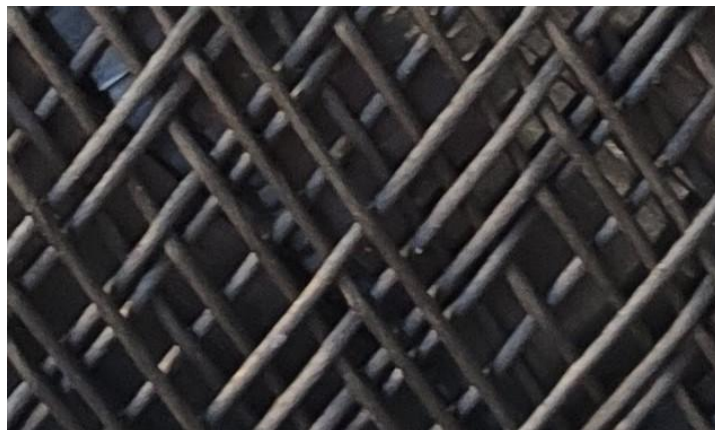
Figure 3.11: Fiber bending and cross sectional deformation during winding
