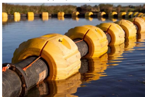
(c) Floating dredging hose
