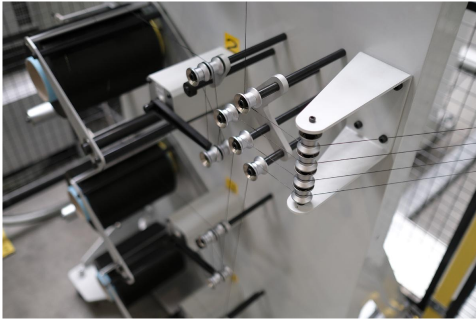
Figure 2.29: Fiber tensioners in the Virgo robot cell
