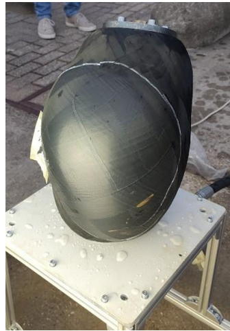
Figure 8.20: Blister formation post burst
