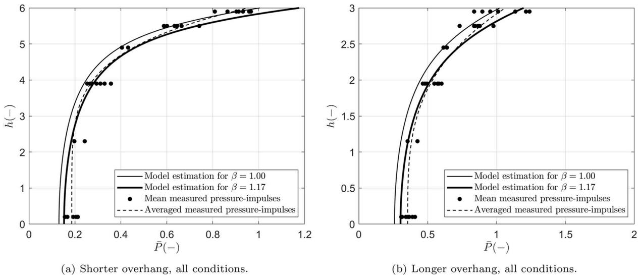
Fig. 15. Summary dimensionless pressure-impulse profile  $\bar{P}$ .
