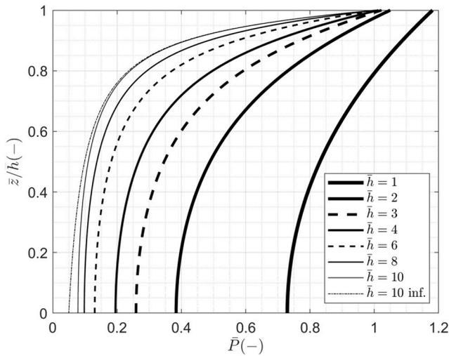
(a) Pressure-impulse profile at wall for  $\beta = 1$ .
