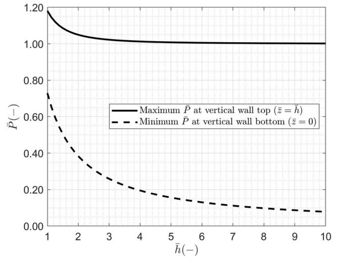
(b) Max and min pressure-impulse at wall for  $\beta = 1$ .
