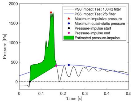
(d) Impact Type IV: for AL and CL. Stepped peak, intermediate vibrations
