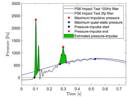
(f) Impact Type VI: for EL and FL. Double peak, intermediate vibrations
