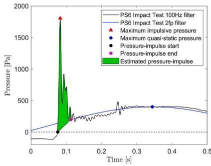
(a) Impact Type I: for AS and CS. Medium peak, intermediate vibrations
