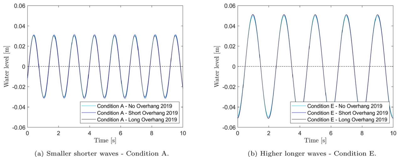
Fig. 11. Example of incident wave time series measured at 1.5 m from the vertical wall.
