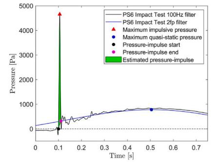
(c) Impact Type III: for ES and FS. Narrow peak, reduced vibrations
