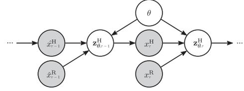
Fig. 4. Bayesian network modeling the robot's intent inference problem. Shaded nodes represent observed variables.
