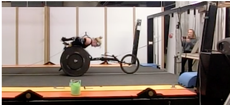
■ Figure 3 Figure 3: Wheelchair racing measurements on a treadmill for sensor-based power estimations.
