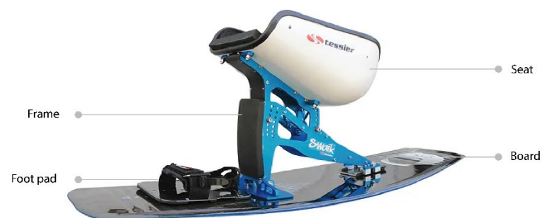
Figure 2: Components of a sitwake
