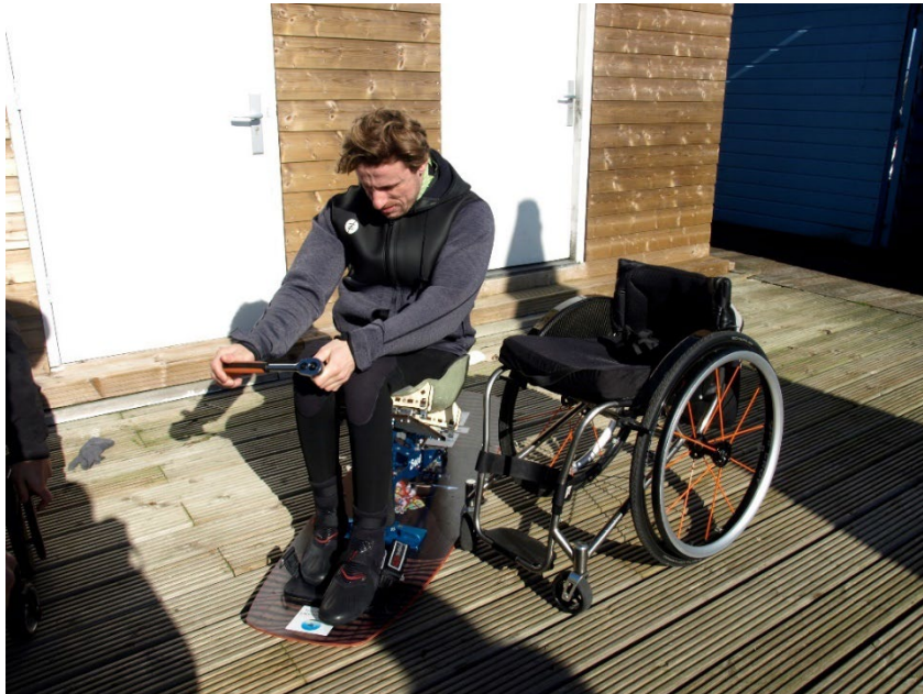
Figure 27: Adjusting the seat with the knob in the front. In this case a ratchet is used.
