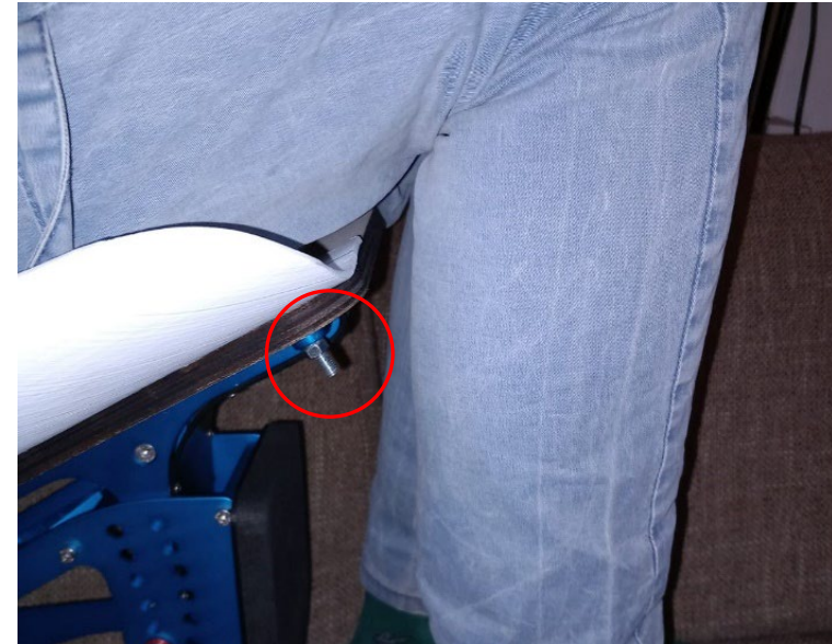
Figure 6c: Bolts causing harm
