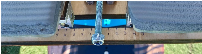
Figure 33: Marks on the base of the first iteration to indicate the size
