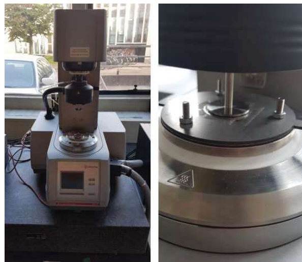
Figure 4: The Anton Paar rheometer MCR 302 used for the experiments and one proof of concept placed in the rheometer.
