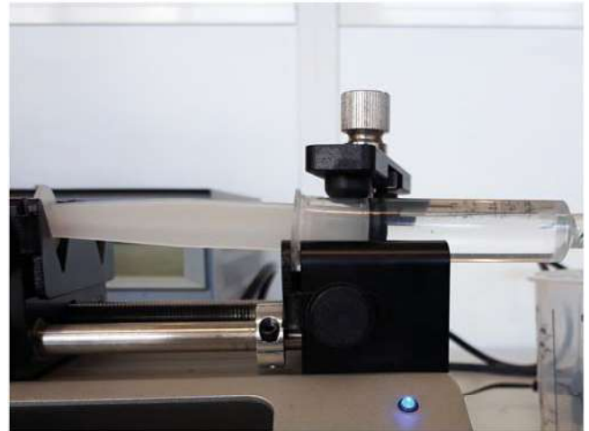
Figure 28. Deformation of the syringe due to high pressure in the system.
