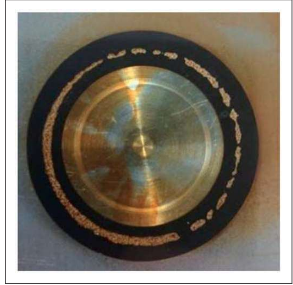
Figure 17. This figure presents the ferrofluid pocket bearing used for the experiment discussed in this section. With a glass plate, the two seals with capillary interconnection are made visible. The magnet used is the HKCM 9963-433.
