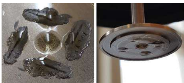
Figure 7: Oil seen on the spindle and laying on top of the magnetic particles after the experiments.
