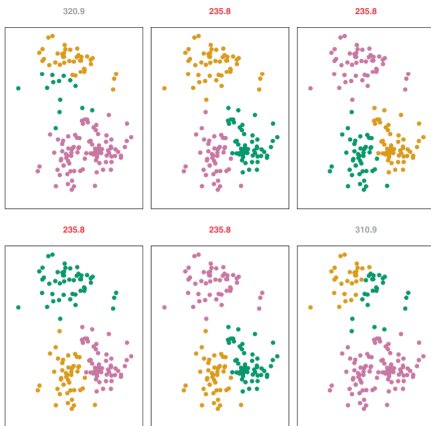
FIGURE 5.2: Six different runs of K-means on the same data set. Different local optimums are reached and the TWSS is displayed above the image. Red numbers indicate the best TWSS (James et al., 2013)
