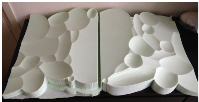
Figure 4.47: Final prototypes, CNC milled from two pieces
