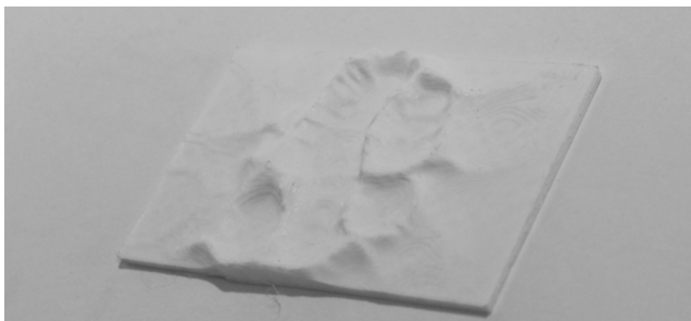
Figure 4.47: Final prototypes, CNC milled from two pieces
