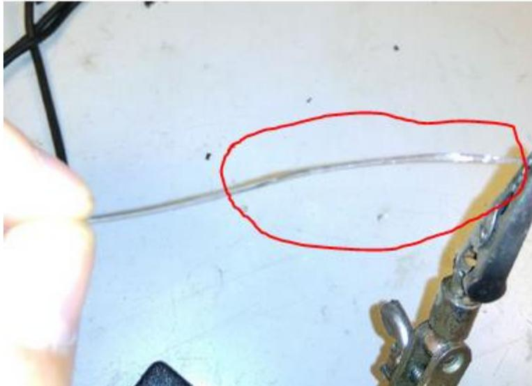
Figure 36. Visible deformation in the fishing wire
