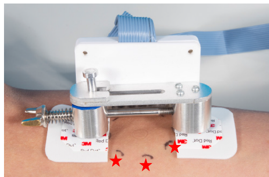
FIGURE 4. Measurement setup during pilot study. Marks (*) indicate where the pads are placed during a single trial. The indications are made on the skin with a mold and marker for direction standardization.
