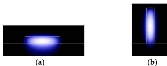
Figure 2. Fundamental mode in: (a) horizontal waveguide and (b) vertical waveguide.
