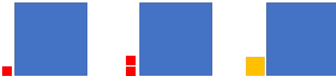
Figure 3.19: Aerial view of building roofs and rainwater harvesting devices. An example to illustrate the concept of (static) effective depth. The blue square is a roof; Small red squares are rain barrels; a medium orange square is a rainwater tank.
