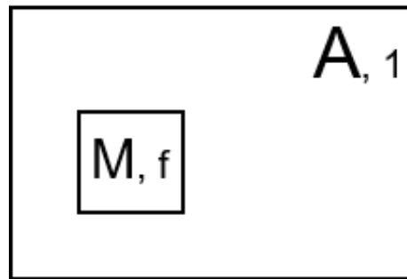
Figure D.17: Illustration of the entire area and the measures inflow area, where A denotes the entire area, the entire area excluding the measure inflow area has the runoff frequency reduction factor of 1, M denotes the measure inflow area, and f is runoff frequency reduction factor over the measure inflow area, which is directly calculated with the Urbanwb Model.
