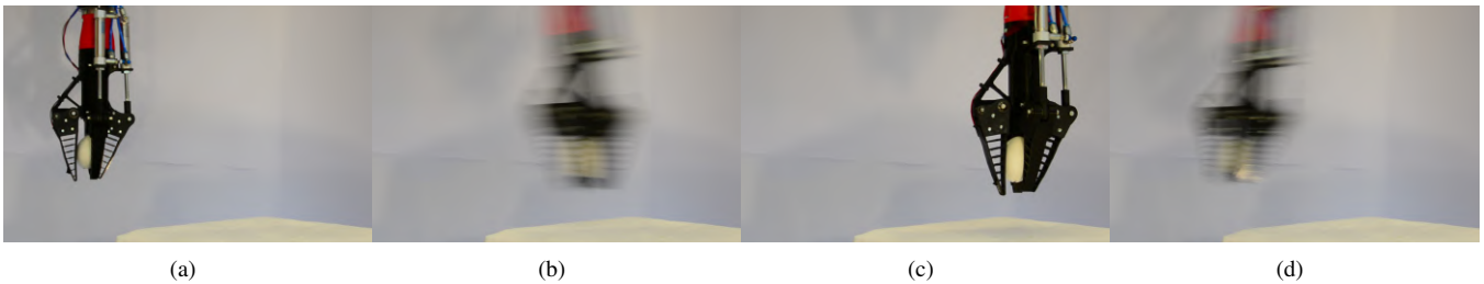
Fig. 10: Snapshots of one back-and-forth cycle of the dynamic holding test, while holding a raw egg. It takes less than 0.4s to execute this motion, which was repeated 40 times without producing any damage to the egg.
