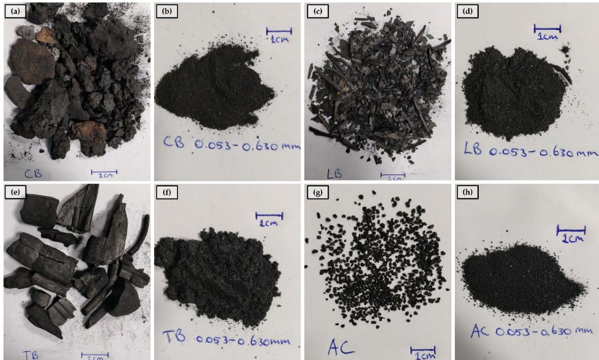
Figure 7. Biochar and activated carbon before and after crushing and sieving procedure. (a-b) Cow dung biochar (CB). (c-d) Jackfruit tree leaves biochar (LB). (e-f) Jackfruit tree branches biochar (TB). (g-h) Activated carbon (AC).
