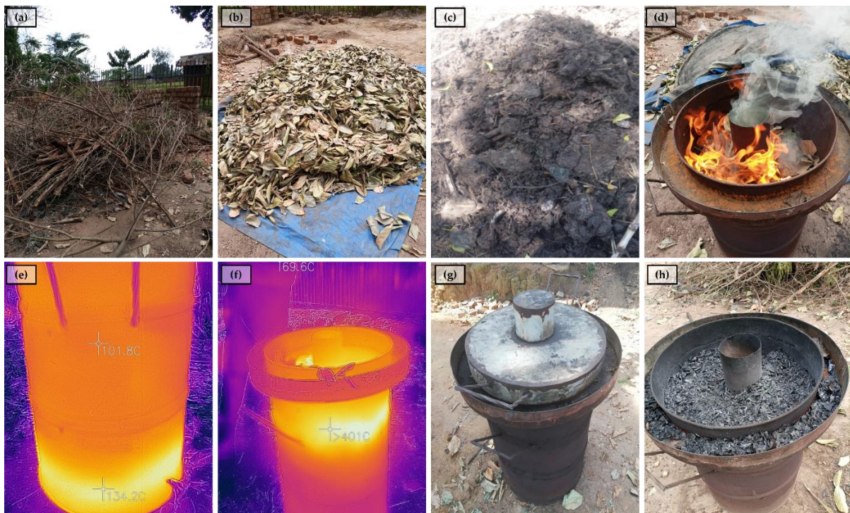
Figure 6. Biochar Carbonization process. (a) Dried jackfruit tree branches. (b) Dried jackfruit tree branches. (c) Dried cow dung. (d-f) Heating up carbonizer to desired 400 °C; measured with a FLIR thermal camera and processed with FLIR Tools software. (g) Carbonization at roughly 400 °C. (h) Finished biochar; biochar made from jackfruit tree leaves in the figure.
