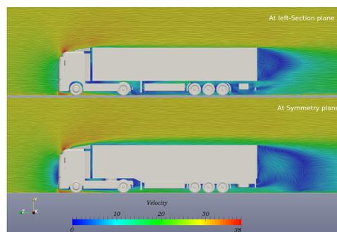
Figure 2.1: Aerodynamic profile for a truck [5]
