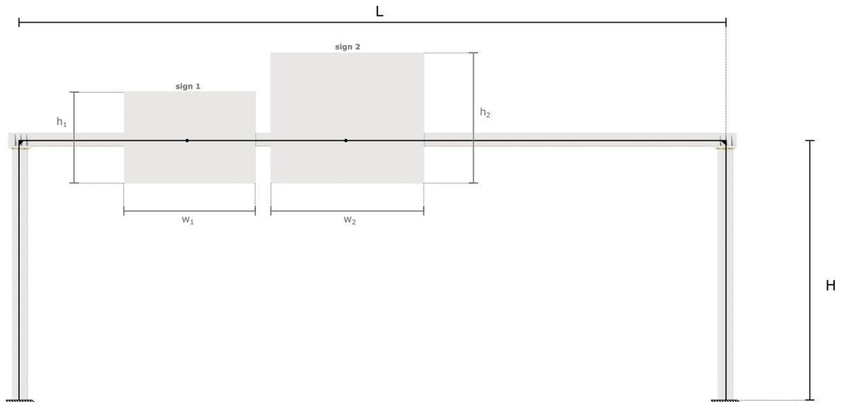
Figure 1.2: Overview of traffic sign support structure
