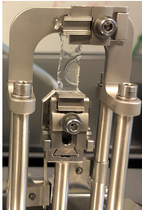
Figure 3.2: Example of the OSTE-PDMS + hydrogel tensile test. Taken from Dynamic Mechanical Analysis tool
