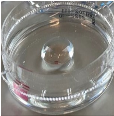
Figure 4.8: Semicured OSTE-PDMS and PEG ODT sample
