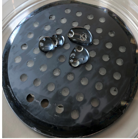
Figure 4.14: Water on the surface of the OSTE-PDMS
