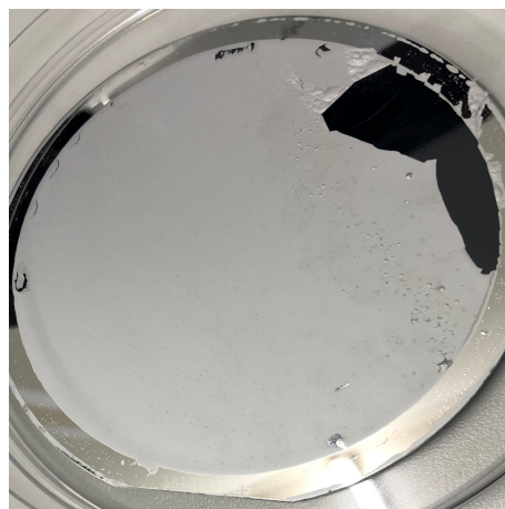
Figure 3.35: Issues caused by degassing o the OSTE-PDMS
