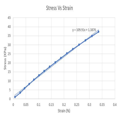
Figure B.8: Stress vs Strain curve OSTE-PDMS
