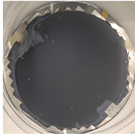
Figure 3.37: Polymer etching after 52 minutes
