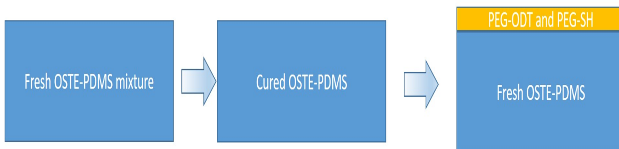
Figure 4.7: Test carried for the bonding of the hydrogel to the OSTE-PDMS surface
