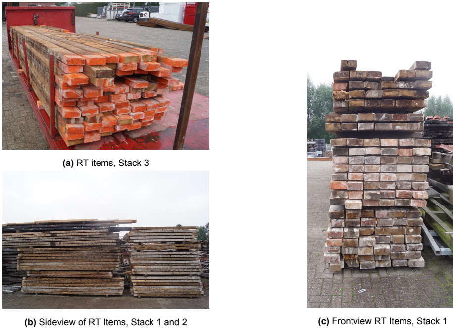
Figure 3.8: Stacks of RT on a Salvage Yard
