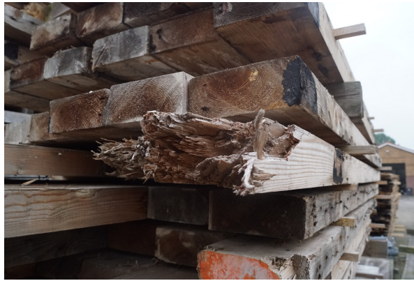
Figure 3.2: Physical Damage due to Demolition, Stack not archived
