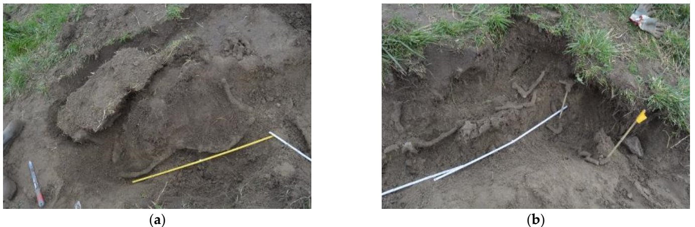
Figure 10. (a,b) Examples of excavated grouted animal burrows.
