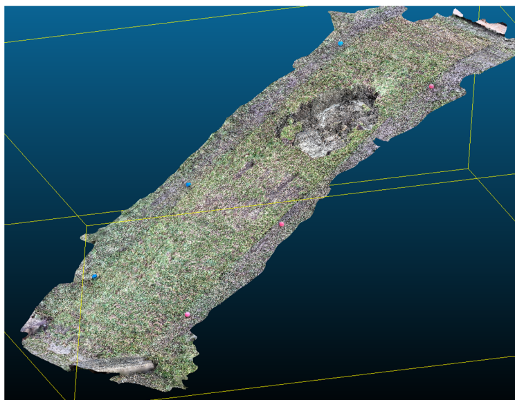
Figure 11. Example of a 3D view of the Handheld Lidar point cloud data of a damaged section.
