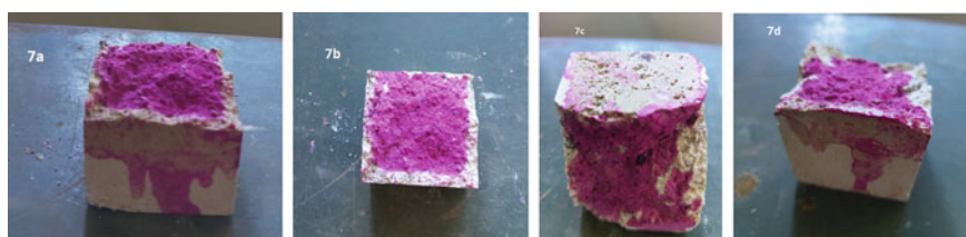
Fig. 7 Carbonation indication on lime mortar samples: a Reference, b with Raisins, c with Dates, d with Zante Currant
