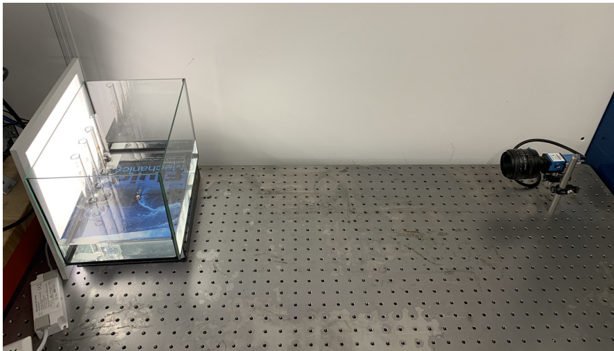
Figure 3.1: Setup of the sedimentation tracking experiments in the lab: the camera is focused on four standing tubes at a distance of approximately 60 cm. The four standing tubes are placed in a container filled with water to match the refractive index with the tubes that contain a water-based suspension with anode or cathode particles. The sedimentation process is tracked by taking pictures of the tube at predetermined time intervals.
