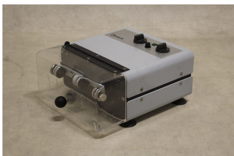
(a) Hertsch MM2 Ball Miller used for grinding the black mass material. At the front, two jars are tightened in the holders, which are horizontally oscillated.
