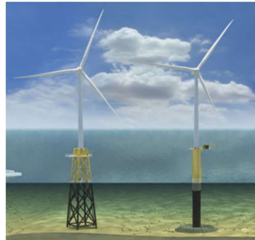
Figure 1-1: Jacket (left) and monopile (right) support structures [5]
