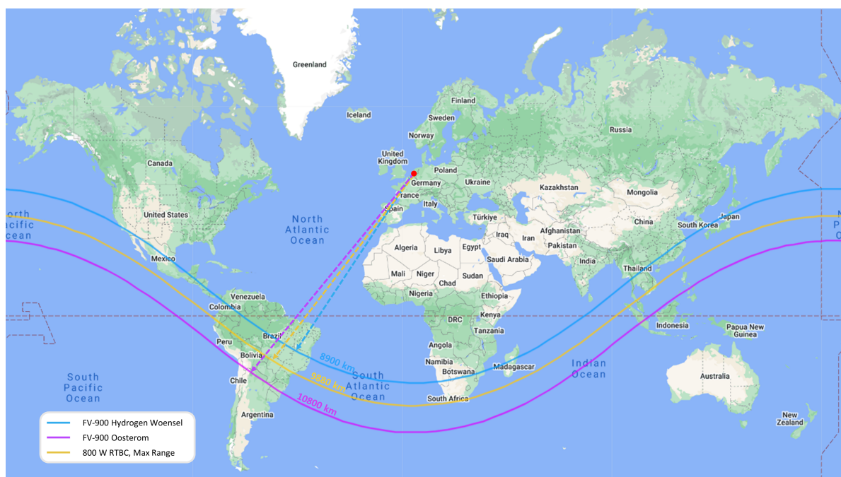
Figure 4.18: The range of three Flying-V concepts at the same Take-off Weight, departing from Schiphol Airport (AMS)
