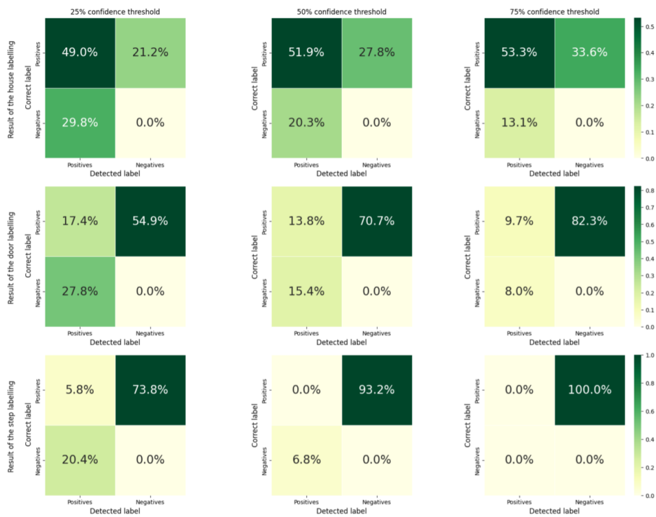
Figure A.1: Nine confusion matrices from the initial. Each column corresponds to confidence thresholds 25%, 50% and 75% and each row represents the classes house, door, staircase, and steps. The true positives are in the top-left corner, the false positives are in the bottom-left corner, the false negatives are in the top-right corner and the true negatives are in the bottom-right corner.
