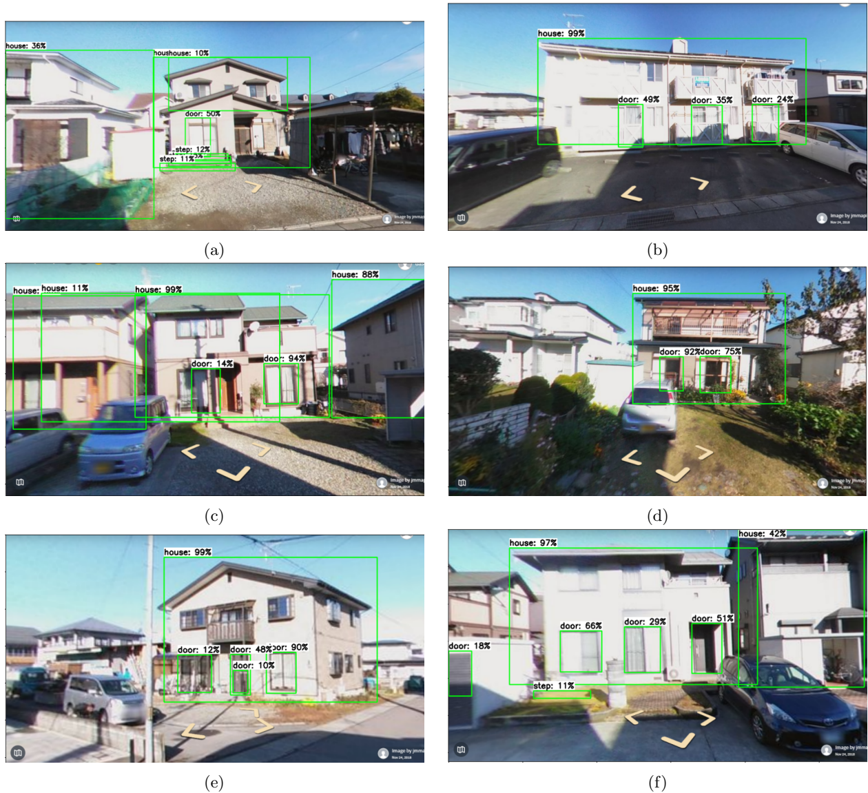
Figure B.2: Six images selected from the problem cases of the predictions of the model where objects were incorrectly labelled as doors. Each bounding box has its corresponding label written directly above with a percentage representing the confidence level of the model.
