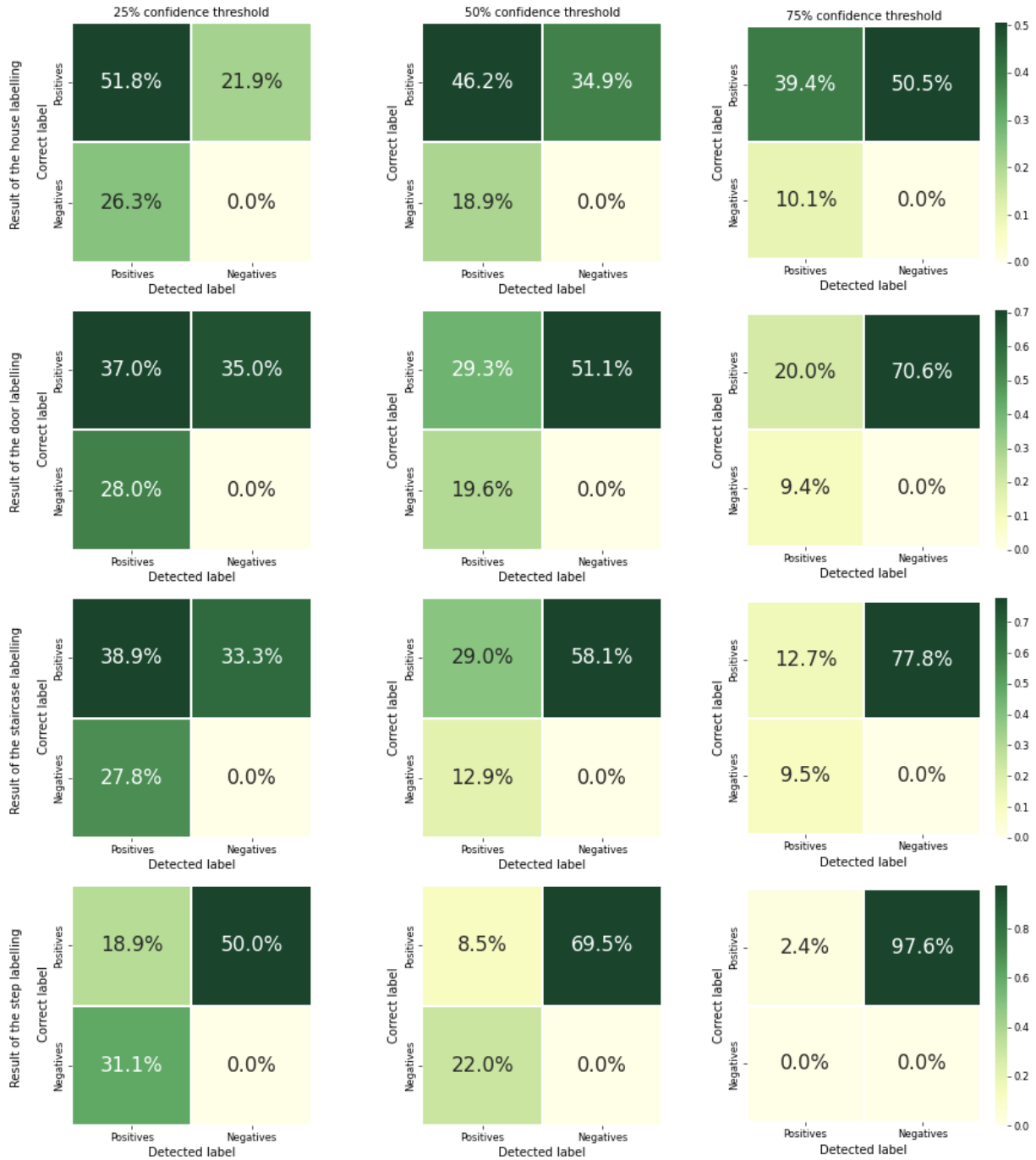
Figure A.2: The confusion matrices for the 'SSD MobileNet v2 FPNLite'-architecture on predicting five classes: house, door, staircase, and steps.
