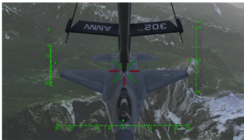
Fig. 2. Experimental setup to do measurements on human control behavior in depth control tasks. (a) The setup comprises a stereoscopic 3D display with two 28-inch monitors, with a semi-transparent mirror in between, and two control sticks. (b) The visual display for a realistic aerial refueling scenario. Here an augmented view is shown, where a target element (red crosshair) is slaved to the receiver aircraft and the controlled element (green crosshair) to the refueling boom in an aerial refueling environment with according information overlay [3, 4]. (c) The visual display used for the pursuit tracking task, where also the target element (red crosshair) and follower marker (green crosshair) are shown on a grey background.
