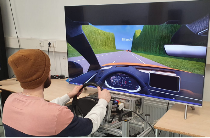
Fig. 1. A participant seated in the fixed-base driving simulator, holding the steering wheel in a ‘ten-to-two’ position. The final on-road obstruction is visible in the distance.
