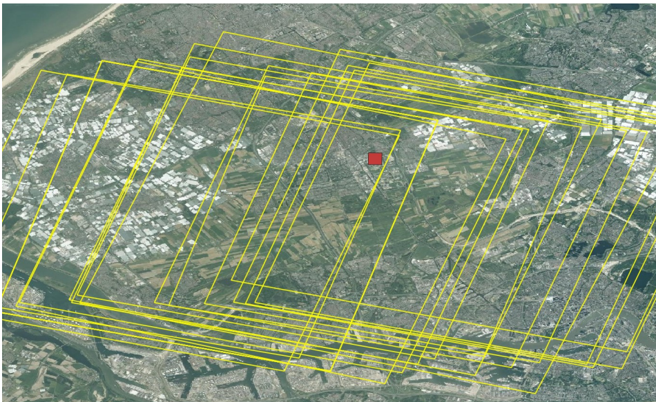
Figure 4.4: Satellite dataset (yellow) visualized on an aerial orthophoto, illustrating the coverage of the SuperView-1 datasets used. The area of interest is marked in red.
