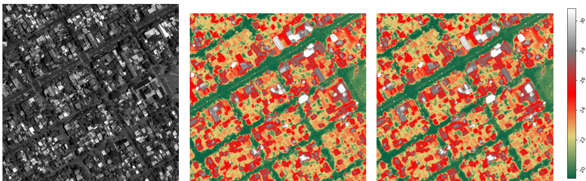
Figure 5.2: From left to right: Input image, initial DEM, adapted DEM, and height [m] color bar for Site 2.
