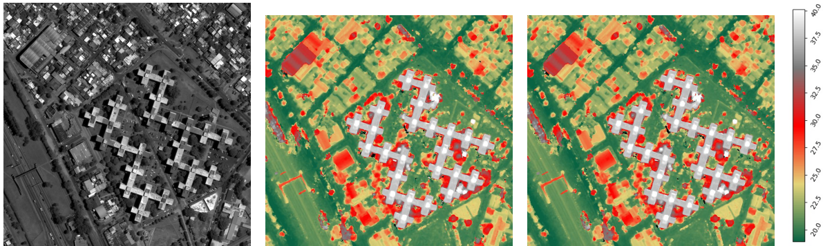
Figure 5.3: From left to right: Input image, initial DEM, adapted DEM, and height [m] color bar for Site 3.
