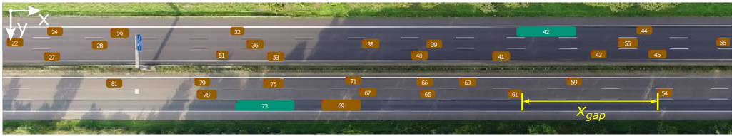
Fig. 4. An example frame of the HighD dataset [17] as visualized using TraViA [39]. The frame includes a stretch of a highway in Germany, where vehicles drive on the right side of the road and where, in some of the cases, there are no legal speed limits. The orange shapes represent regular cars, the green shapes are trucks. All vehicles have a vehicle-ID shown in white. The white arrows display the coordinate frame and the yellow marking shows a visualization of the gap between two vehicles as used in the metrics for step 3 of the validation workflow.
