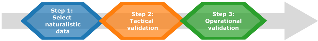
Fig. 2. The proposed driver model validation workflow for interaction-aware autonomous vehicle controllers. The workflow consists of three steps. In the first step, a suitable dataset is selected to perform the validation of the driver model on. From this selected dataset, specific situations are automatically extracted. The actual validation of the model takes place in the last two steps. A distinction is made based on the level of behavior. First, the tactical behavior is validated in step 2. This step reveals to what extent the driver model shows tactical behavior that is consistent with human behavior in the dataset. Behavior inconsistent with human data, e.g., collisions, is not regarded in the final step. The third step evaluates the operational behavior of the model based on human-factors literature. This is done for every tactical behavior separately. The final conclusion of the validation should be based on the combined results of steps 2 and 3.
