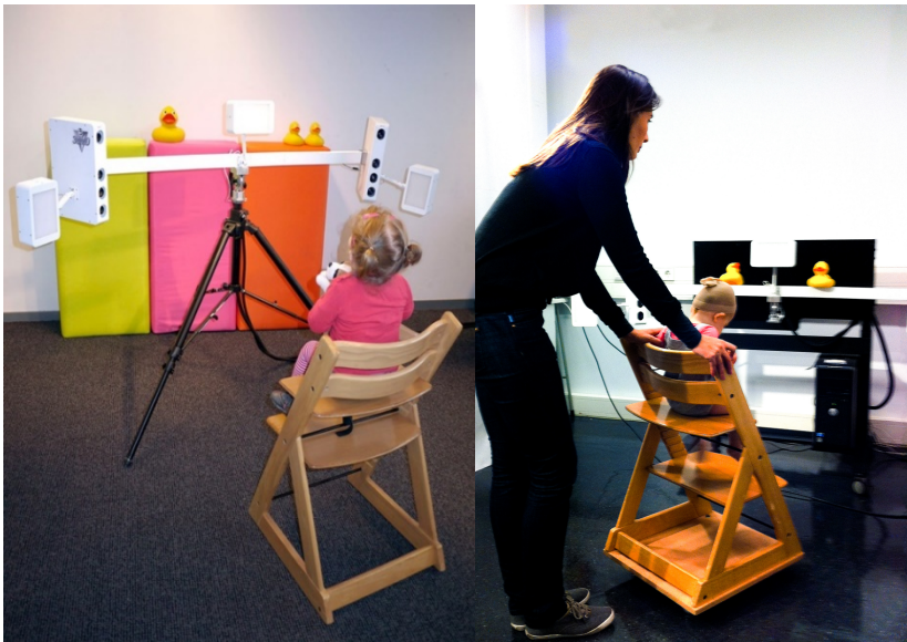
Figure 8 3D imaging setup with a 3-year-old girl (left) and with a 1-year-old girl sitting on the highchair mounted on the wheeled plateau (right).
