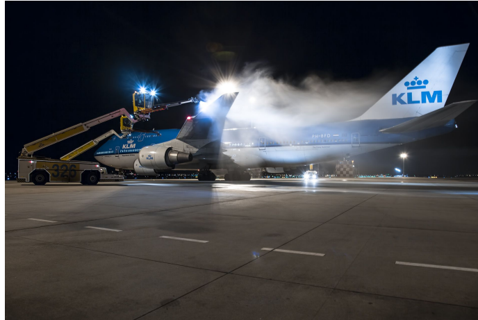
Figure 3.5: De-icing of an aircraft (Schiphol, 2019a)
