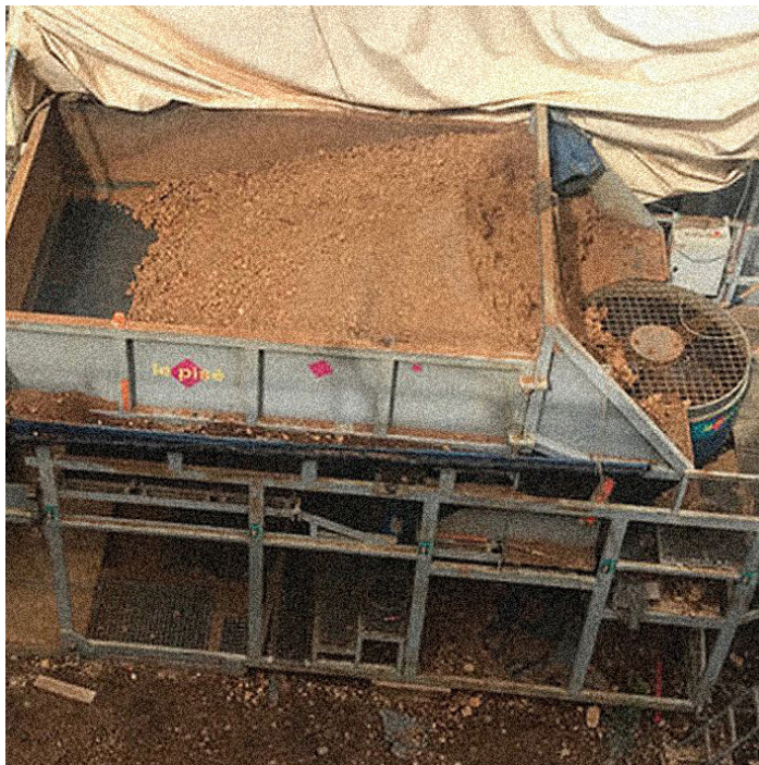
Figure 33 The raw material is stored on top of the station and is transferred towards a mixer with a sieve on top.
