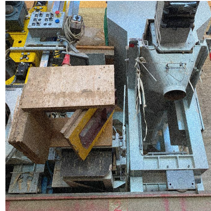
Figure 16 The outlet for rammed earth material, which is centred above the formwork.
