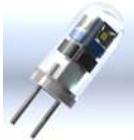
Fig. 5.3 Proposed G4 retrofit LED prototype (Schematic drawing)
