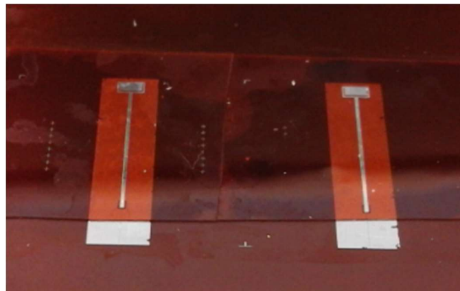
Fig. 6.15: The final device attached with primer, aligned by self designed alignment marks
