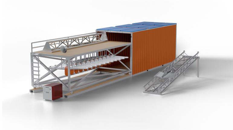
Figure 73: Artistic visualisation of the ground system with the rail and backup generator already dismantled
