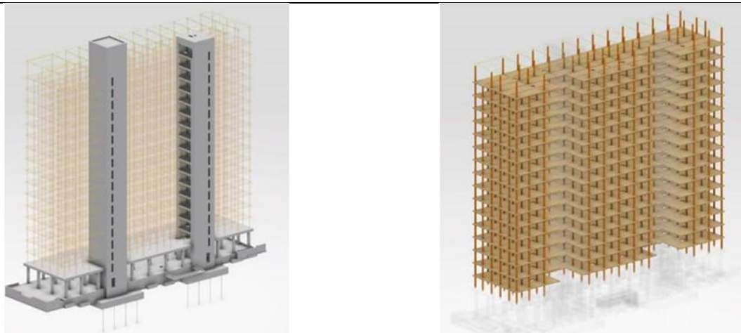
figure 1-2: Overview of the Brock Commons structural system. Left: Concrete platform and cores. Right: Timber pendulum structure (Fast, Gafner, Jackson, & Li, 2016).
