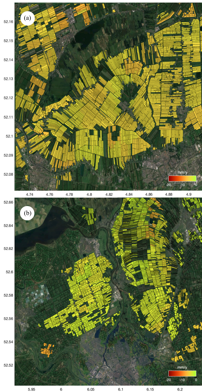
Fig. 10. Color-coded map of estimated linear subsidence rates for the period January 1, 2017–December 31, 2022, at (a) Zegveld and (b) Rouveen regions. Parcels with no fill indicate that no estimation has been made at that location.
